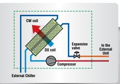
The "Dual Cooling" version is equipped, in addition to the DX evaporating coil, with a CW coil receiving chilled water by, for instance, a chiller. In this way, the requested cooling capacity can be delivered even in case of malfunction of the main refrigerating circuit, guaranteeing the system the maximum redundance possible.
