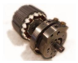
The Brushless synchronous motor has "no brushes" as the power is only sent to the stator and not directly to the rotor, therefore, sliding electrical contacts are not required. Over 20 Hz, the mP on board controls a feedback signal (BEFM Back Electro Motrice Force) that can certify the rotor's synchronous rotation with a magnetic field and implements any torque corrections to restore/maintain synchronism and therefore maximum efficiency.
